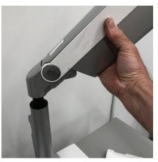
13 Install the new M8 Long Dynamic arm, making sure the plastic washer stays on the dynamic arm link pin as it slides into the QSL base socket.
