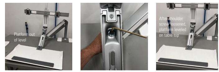
16 Once the platform is lying flat in the desired position, tighten the bolt as tight as possible with 5mm Allen Key. **If available, use a torque wrench and tighten to 15 ft. lbs.**
