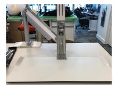
OSL platform leveled with bolt fully tightened
