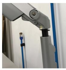
14 Reinstall QSL head, making sure that the plastic link washer stays in place on the link pin as it is inserted into the dynamic arm socket. Re-tighten set screws on either end of the dynamic arm. Position the QSL keyboard platform on a flat desk or work surface.
