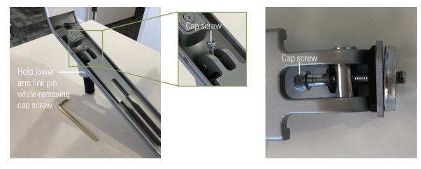
6 Continue loosening this screw until it can be removed from the unit. Remove the cap screw with the release lever, and all washers that the screw passes through. Remove the arm link pin, which will be replaced in the upgrade process. QSL head assembly is now resting on the work surface ready to be reassembled with the replacement parts.
